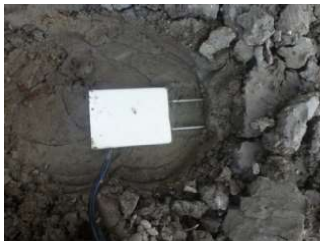
Figure 13 Placement of TDRs
