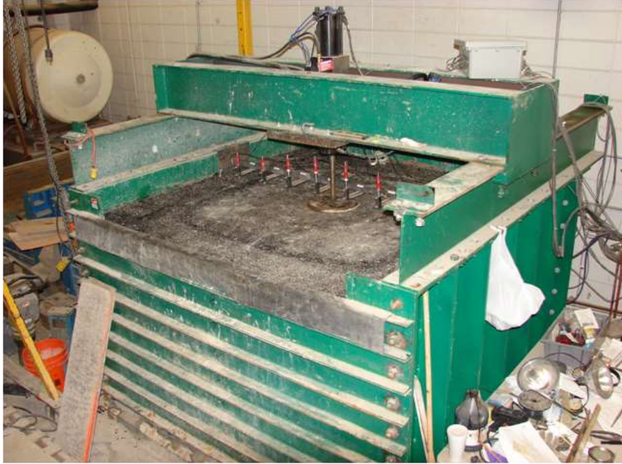
Figure 20 Image of the indoor cyclic plate load test facility
