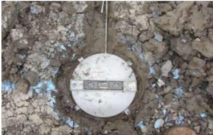
Figure 12 Placement of pressure cells
