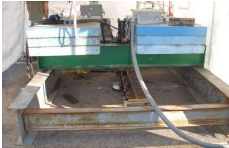
Figure 17 In-field cyclic plate load testing facility
