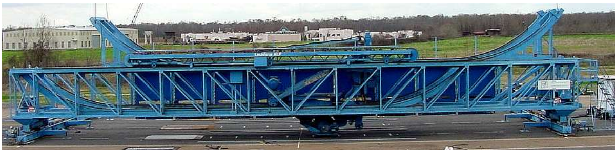
Figure 16 Moving wheel load testing facility
