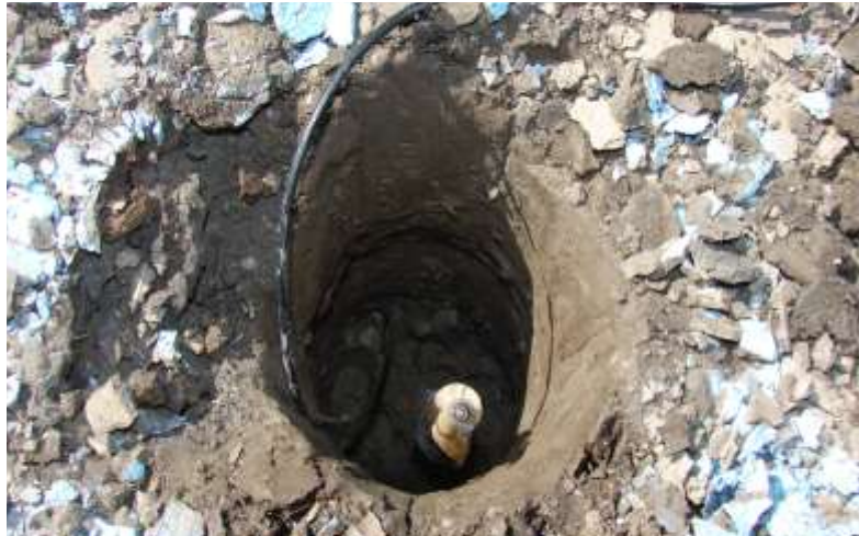
Figure 10 Placement of LVDTs
