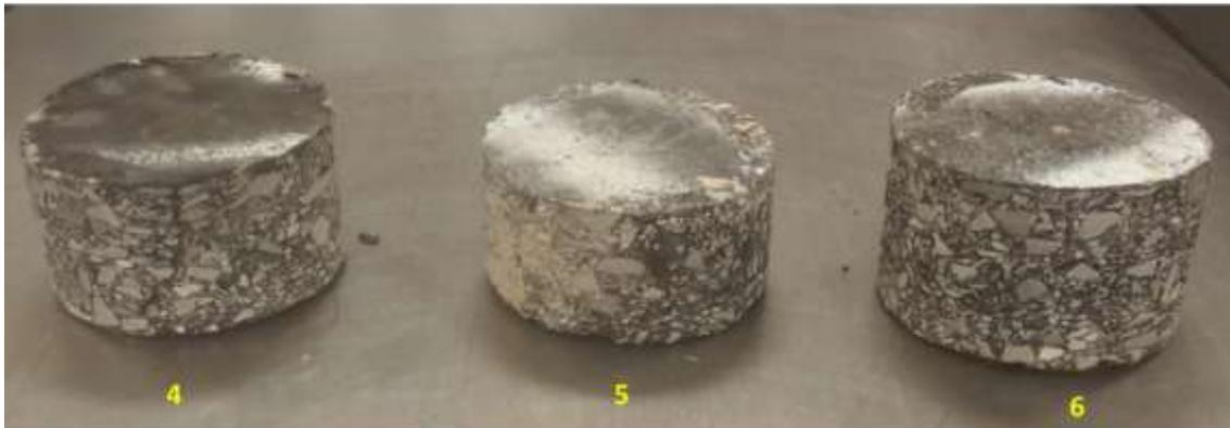
**(b) Cores from sealed section**
