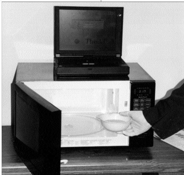
The results of this study will validate the accuracy of microwave ovens in the determination of moisture contents under both field and laboratory conditions.
