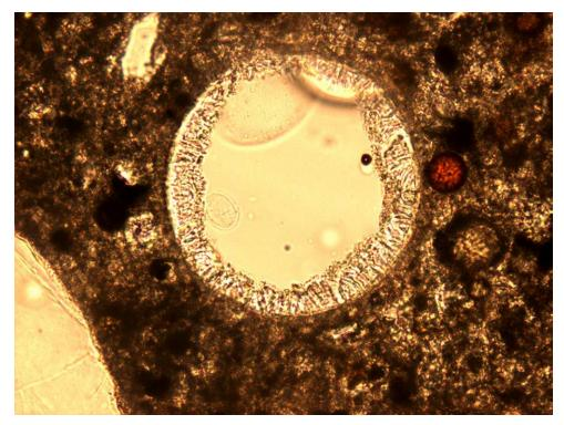
Figure A1-7: Another image of ettringite in an air void. Width of field is 0.33 mm. Thin section image.
