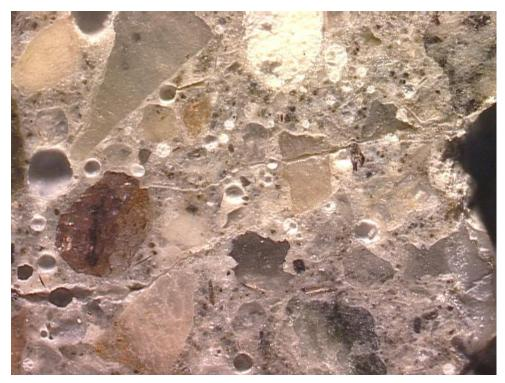
Figure G1-9: Cracks that are found just below the exposed surface. Width of field is 4.0 mm. Polished surface section image. The exposed surface is on the right side.
