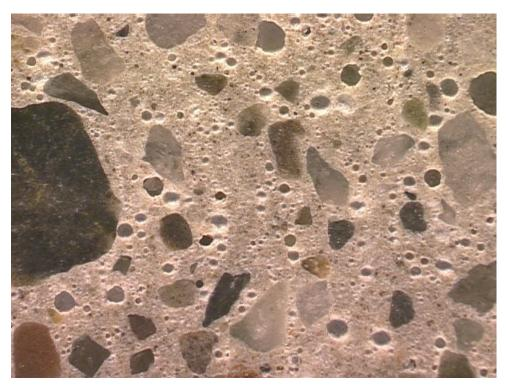
Figure S1-3: Entrained air voids in the concrete. Width of field is 4.0 mm. Polished surface image.
