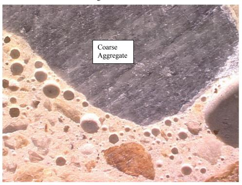
Figure Q1-4. Another image of air voids surrounding coarse aggregate. Width of field is 6.5 mm. Polished surface image.
