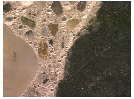
Figure S1-4: The bonding between aggregate and cement paste is good. Width of field is 4.0 mm. Polished surface image.
