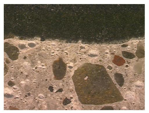
Figure S1-9: Cracking at the interfacial region between the paste and coarse aggregate. Width of field is 4.0 mm. Thin section image.
