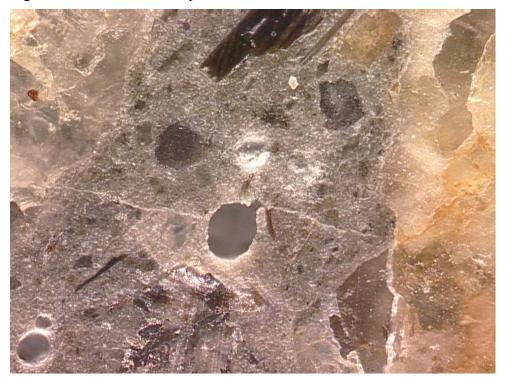
Figure F1-8: A crack connecting two aggregate pieces. Width of field is 2.0 mm. Polished surface image.
