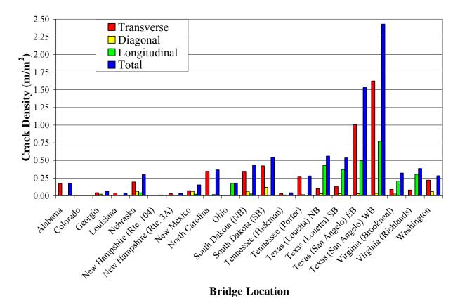
Figure 20. Chart. Crack Densities for All Bridge Decks.
