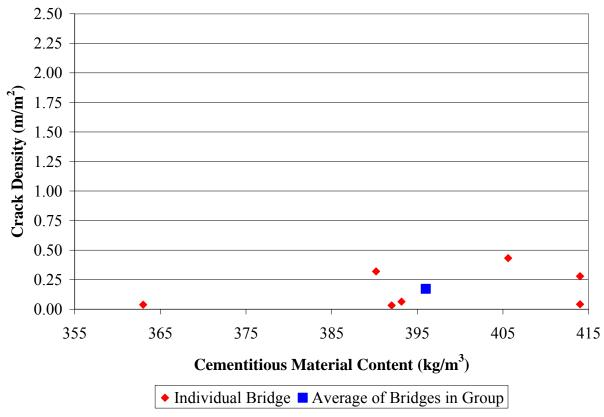
Figure 26. Chart. Crack Densities for Cementitious Material Contents between 356 and 415 kg/m<sup>3</sup> (600 and 700 lb/yd<sup>3</sup>).
