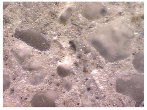
Figure C1-4: The bonding between aggregate and cement paste is moderate. Width of field is 2.0 mm. Polished surface image. Note a crack is at the center of the image.
