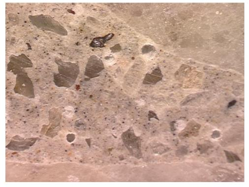
Figure A1-4: The bonding between aggregate and cement paste is strong. Width of field is 4.0 mm. Polished surface image.
