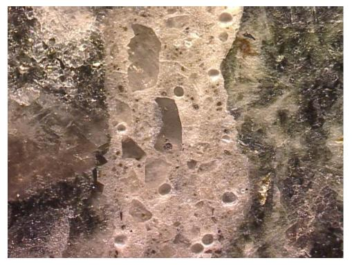
Figure G1-5: The bonding between aggregate and cement paste is strong. Width of field is 4.0 mm. Polished surface image.
