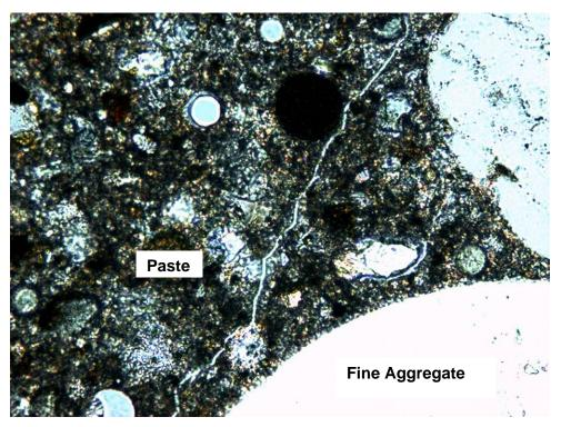
Figure P1-7. Crack in the cement paste and close to the aggregate/paste interface. Width of field is 0.33 mm. Thin section image.
