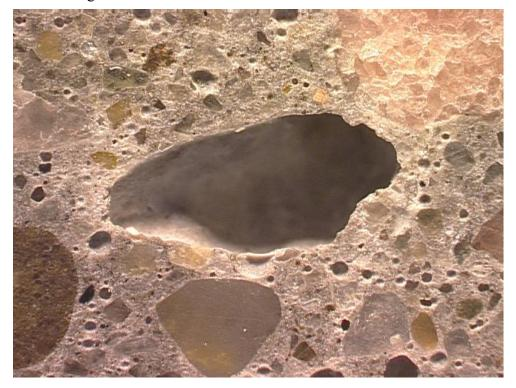
Figure K1-6: An entrapped air void. Width of field is 6.5 mm. Polished surface image.
