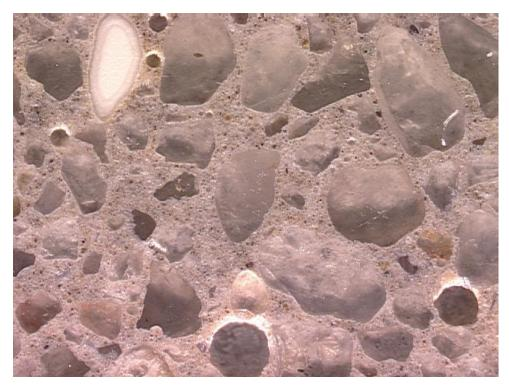
Figure O1-5: Another view of the air voids in the concrete. Width of field is 4.0 mm. Polished concrete surface image.
