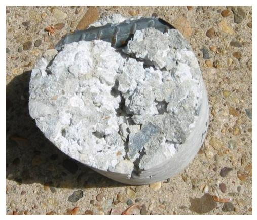
Figure A1-9: Honeycombing in core AL-5.
