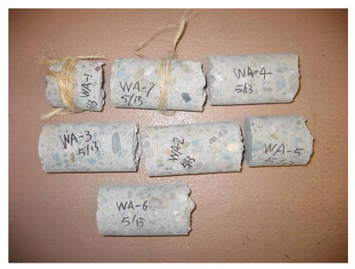
Figure S1-1: Seven concrete cores as received.
