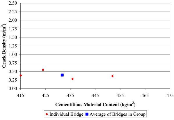
Figure 27. Chart. Crack Densities for Cementitious Material Contents between 415 and 475 kg/m³ (700 and 800 lb/yd³).
