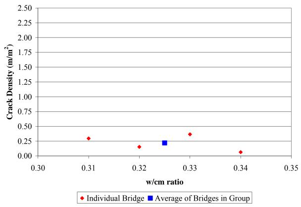
Figure 22. Chart. Crack Densities for w/cm ratio 0.30 to 0.35.
