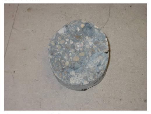
Figure J1-2: Honeycombing in core OH-6.
