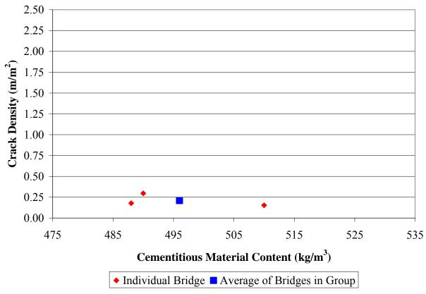
Figure 28. Chart. Crack Densities for Cementitious Material Contents Greater than 475 kg/m³ (800 lb/yd³).
