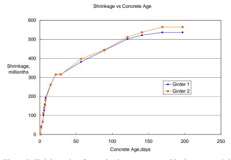
Figure 2. Shrinkage data for production concrete used in the precast girders.
