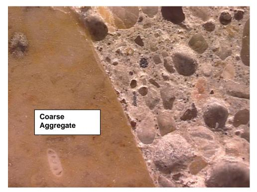
Figure P1-10. Gap between the coarse aggregate and the paste. Width of field is 4.0 mm. Polished surface image.
