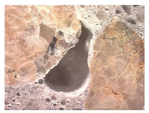
Figure I1-5: An entrapped air void between two aggregate particles. Width of field is 4.0 mm. Polished surface image.
