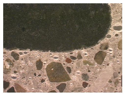
Figure S1-5: A gap has formed between the aggregate and paste. Width of field is 6.5 mm. Polished surface image.
