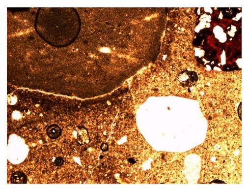
Figure J1-7: Cracks around aggregate as well as in paste. Width of field is 0.16 mm. Thin section image.
