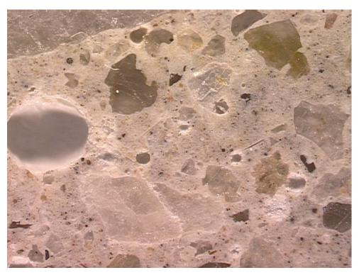
Figure A1-3: Entrained air voids in the concrete. Width of field is 4.0 mm. Polished surface image.
