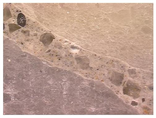
Figure A1-5: Another image showing the aggregate-paste interface is dense and strong. Width of field is 4.0 mm. Polished surface image.
