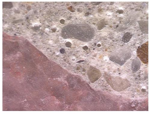
Figure L1-4: The bonding between aggregate and cement paste is moderately strong. Width of field is 2.0 mm. Polished surface image.
