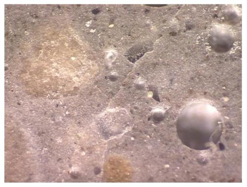
Figure J1-9: Cracks as seen in the polished slab. Width of field is 1.1 mm.
