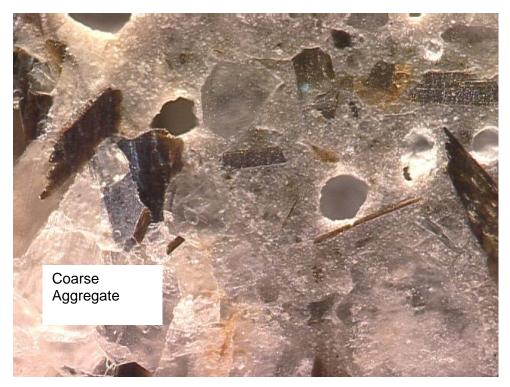
Figure F1-5: The bonding between aggregate and cement paste is strong. Width of field is 2.0 mm. Polished surface image.
