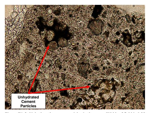
Figure E1-2: Unhydrated cement particles in the paste. Width of field is 0.33 mm, thin section image.
