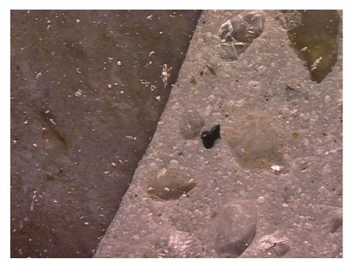
Figure M1-7: An image of aggregate/paste interface. Width of field is 2.0 mm. Polished surface image.
