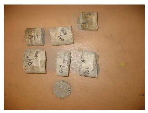
Figure J1-1: Seven cores as received. Notice that the small piece at the bottom (OH-4) is a 7/8-in. thick disc.
