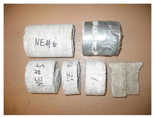
Figure E1-1: Six concrete cores as received.
