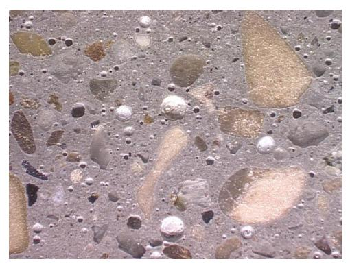
Figure J1-5: The bonding between aggregate and cement paste is moderate to poor. Width of field is 6.5 mm. Polished surface image.
