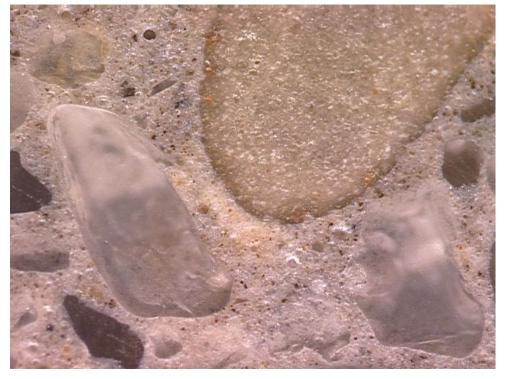
Figure O1-10: Paste/fine aggregate interfacial region. Width of field is 2.0 mm. Thin section image.
