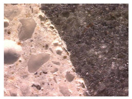
Figure R1-5: Gaps and voids in the paste/coarse aggregate interfacial region. Width of field is 2.0 mm. Polished surface image.
