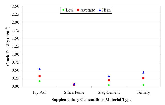
Figure 29. Chart. Crack Density for Supplementary Cementitious Materials.
