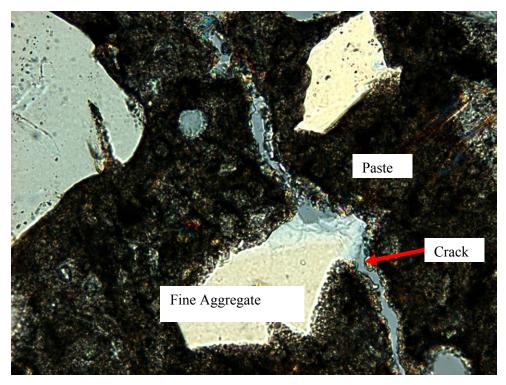
Figure Q1-7. Crack in the cement paste and along the aggregate/paste interface. Width of field is 0.33 mm. Thin section image.
