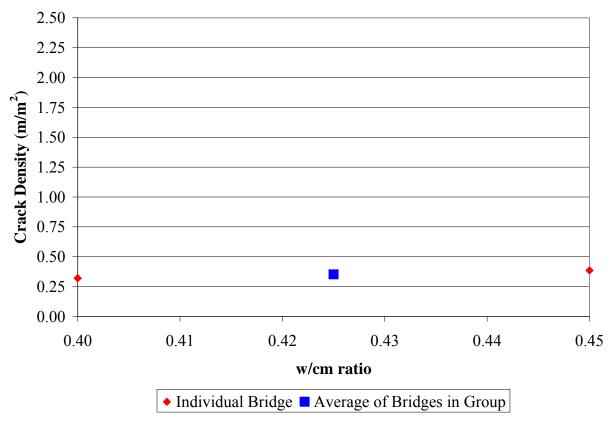
Figure 24. Chart. Crack Densities for w/cm ratio 0.40 to 0.45.
