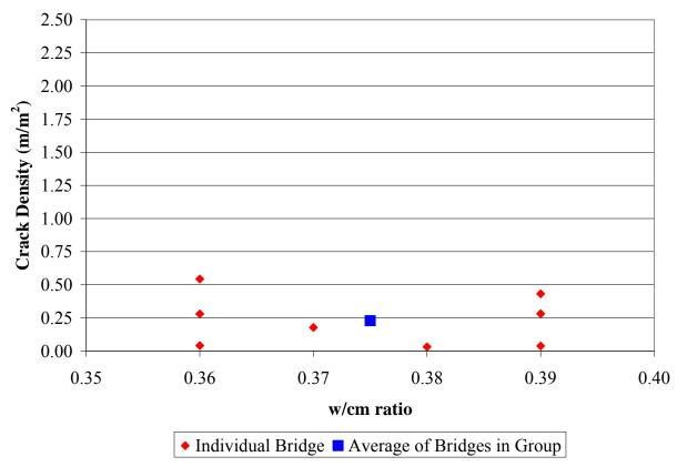
Figure 23. Chart. Crack Densities for w/cm ratio 0.35 to 0.40.
