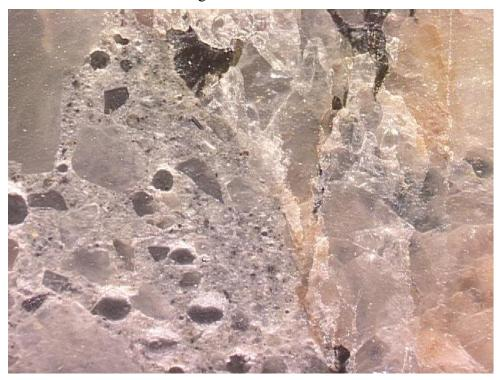
Figure I1-7: The bonding between aggregate and cement paste is good. Width of field is 4.0 mm. Polished surface image.
