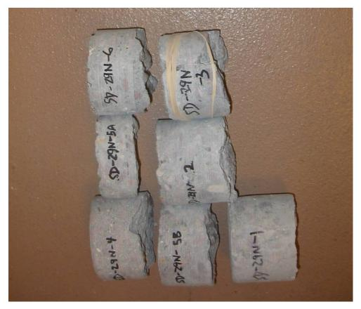
Figure K1-1: Seven concrete cores as received.
