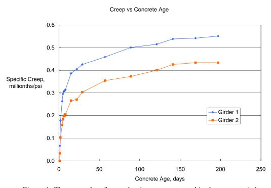
Figure 1. The creep data for production concrete used in the precast girders.
