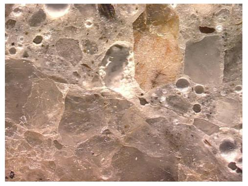
Figure G1-8: Crack in the aggregate-paste interfacial region. Width of field is 4.0 mm. Polished surface image.
