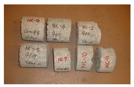
Figure I1-1: Seven concrete cores as received.
