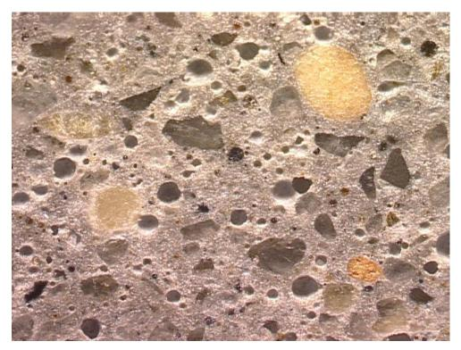
Figure K1-5: Entrained air voids in the concrete. Width of field is 4.0 mm. Polished surface image.
