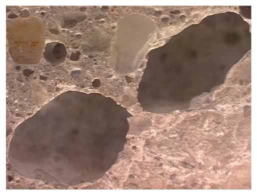
Figure E1-5: Two entrapped air voids. Width of field is 6.5 mm, polished surface image.
