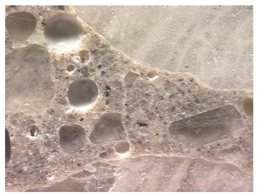
Figure E1-9: A crack in the paste between two aggregate particles. Width of field is 2.0 mm, polished surface image.
