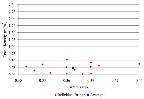
Figure 21. Chart. Crack Density vs. w/cm ratio for all Bridge Decks.
