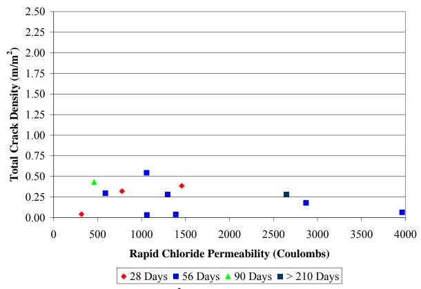
Figure 30. Total Crack Density (m/m²) versus Rapid Chloride Permeability (Coulombs).
