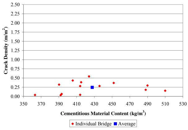
Figure 25. Chart. Crack Density vs. Cementitious Material Content for all Bridge Decks.
