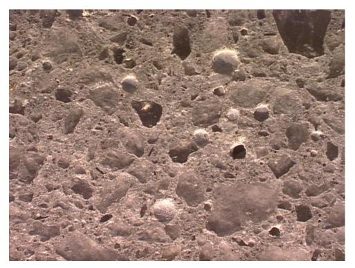
Figure C1-3: Entrained air voids in the concrete. Width of field is 6.5 mm. Polished surface image.
