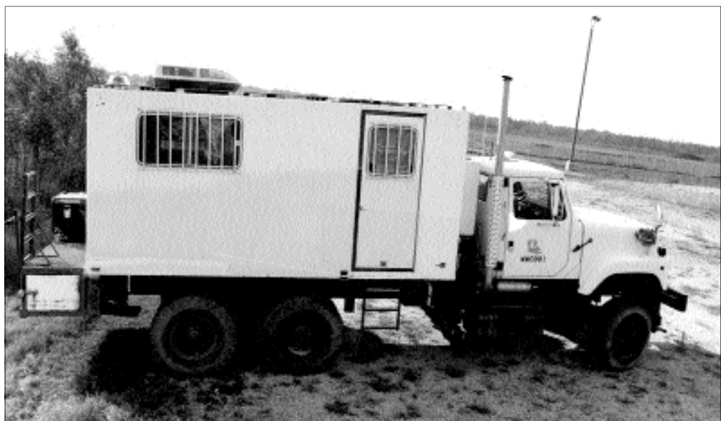
The LTRC electronic cone penetrometer truck to be used in the evaluation of the bearing capacity of piles.
