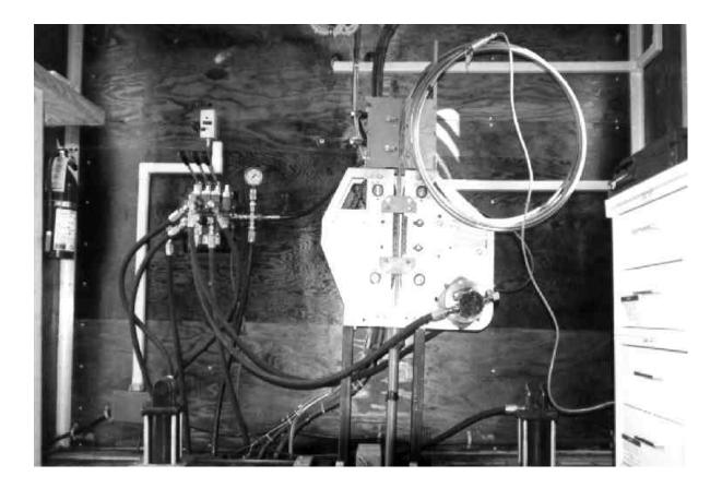
Figure 5 The cone penetration test systems used in the study, the caterpillar-type continuous push device of the CIMCPT system.
