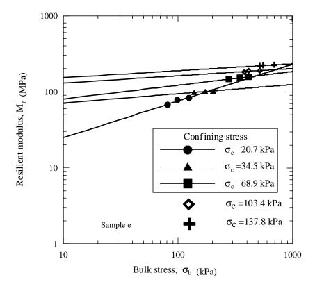
Figure 20 Variation of the resilient modulus with bulk stress at different confining pressures for Larose sand
