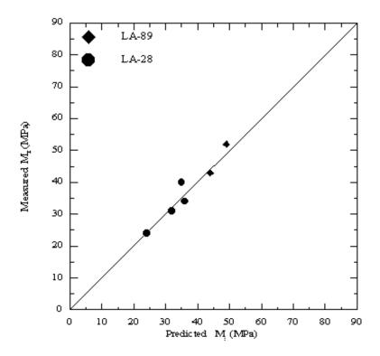
Figure 25 Predicted versus measured resilient modulus of the investigated cohesionless soils.
