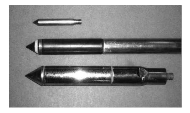
Figure 6 Miniature versus 10 and 15 cm<sup>2</sup> cone penetrometers.
