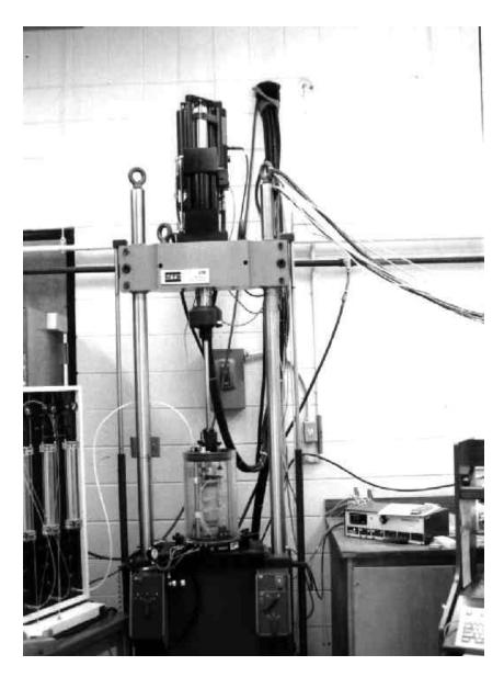
Figure 10 Photograph showing the triaxial cell and control panel.
