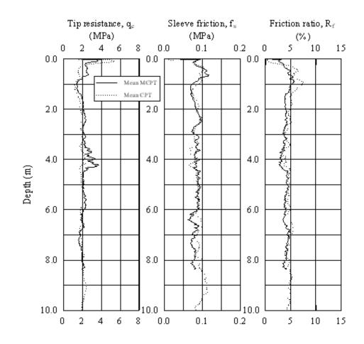
Figure 17 Statistical analysis for the MCPT and CPT soundings at Highland Road site. (a) Comparison of means of MCPT and CPT tests on Highland Road clay.
