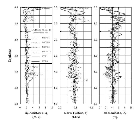
Figure 16 CPT and MCPT tests at the LA-42 test site (test set 1).
