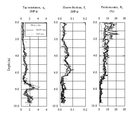
Figure 14: (a) Cone penetration tests (MCPT and CPT soundings) on the heavy clay.
