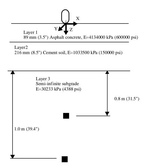
Figure 22 A typical pavement section for traffic stress analysis.
