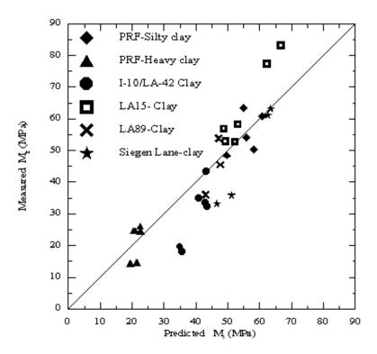
Figure 23 Prediction of in situ resilient modulus by cone penetration test results
