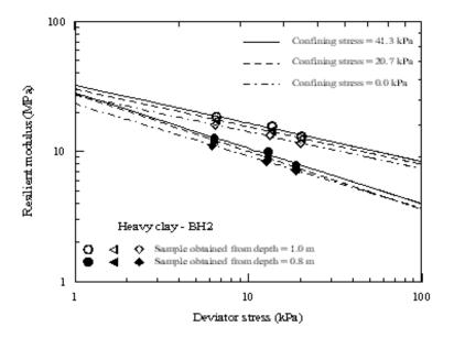
Figure 19 (b) Variation of the resilient modulus with deviator stress at different confining pressures for heavy clay obtained from borehole BH2
