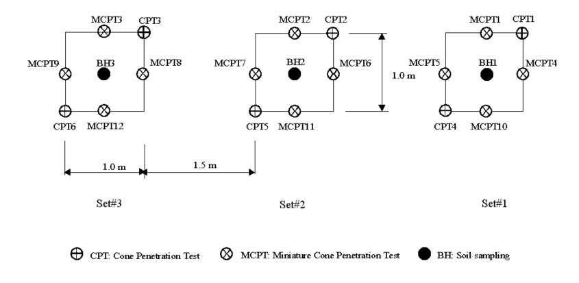
Figure 7 A typical field testing layout for the soil at a selected test site.
