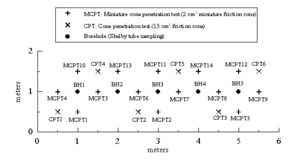
Figure 15 Field testing plan at the (a) I-10 @ Highland Road (LA State Route 42) test site
