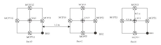
(a) Field tests on the PRF-silty clay.
