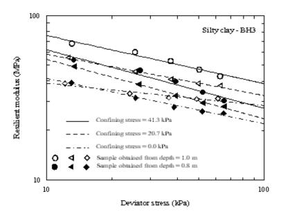
Figure 18 (c) Variation of the resilient modulus with deviator stress at different confining pressures for silty clay obtained from borehole BH3
