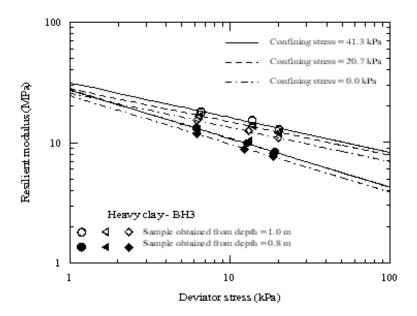
Figure 19 (c) Variation of the resilient modulus with deviator stress at different confining pressures for heavy clay obtained from borehole BH3
