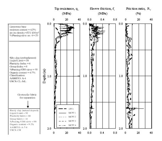
Figure 13: (a) Cone penetration test results (MCPT and CPT soundings) on the silty clay % f(x) = 0
