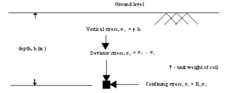
Figure 21 Estimation of in situ resilient modulus from the laboratory resilient modulus test results
