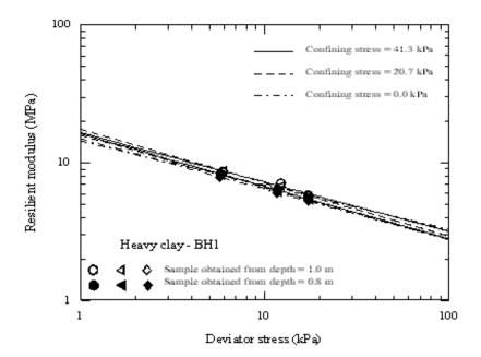
Figure 19 (a) Variation of the resilient modulus with deviator stress at different confining pressures for heavy clay obtained from borehole BH1
