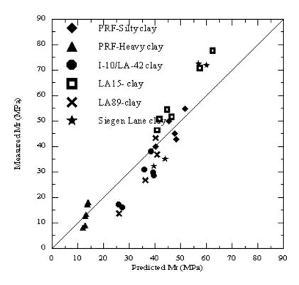
Figure 24 CPT-Resilient modulus of cohesive soil under traffic loading
