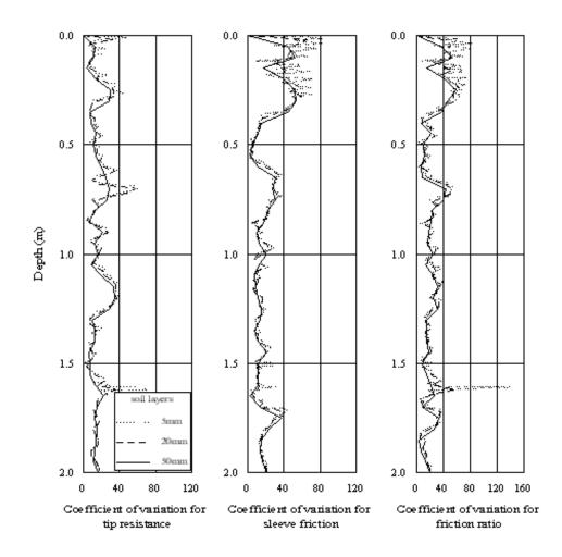
Figure 13: (b) Statistical analyses of the MCPT soundings on silty clay (set 1).
