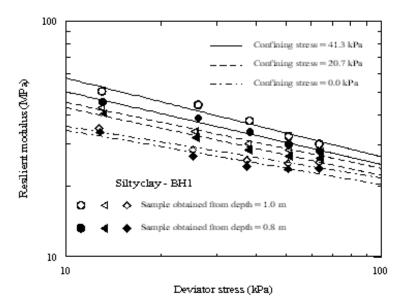
Figure 18 (a) Variation of the resilient modulus with deviator stress at different confining pressures for silty clay obtained from borehole BH1
