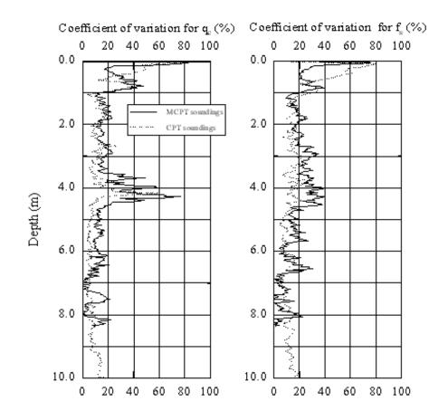
Figure 17 Statistical analysis for the MCPT and CPT soundings at Highland Road site. (b) Comparison of COV profiles with depth for the MCPT and CPT tests.
