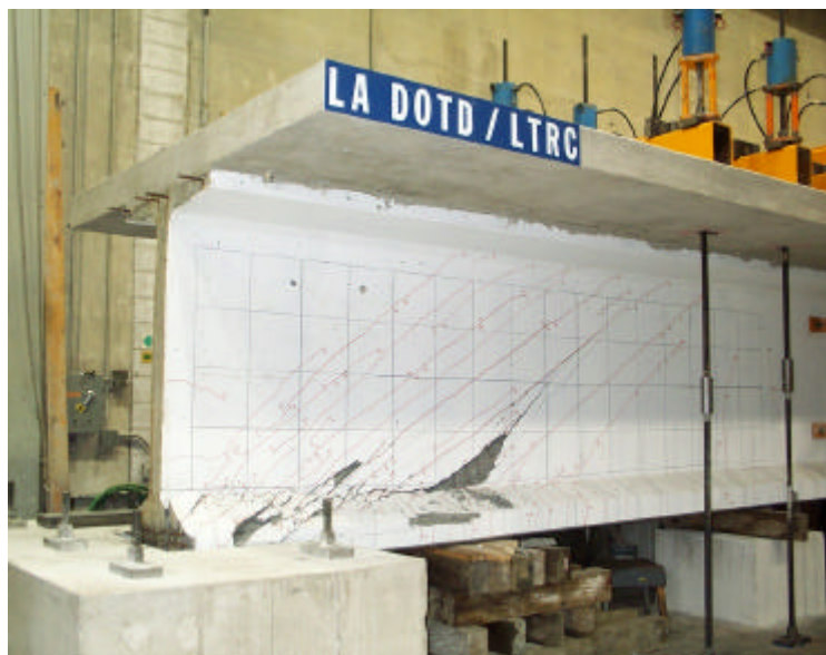
Figure 16 Specimen BT8-Dead after the shear test
