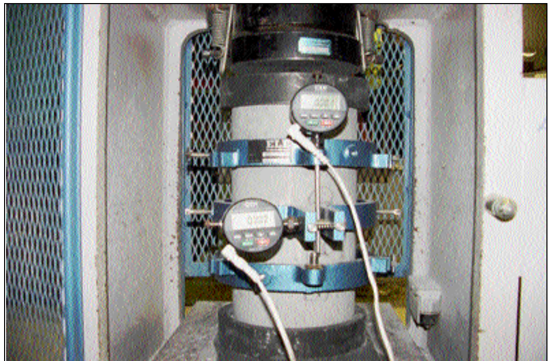
A modulus testing frame with a 6 x 12 cylinder.
