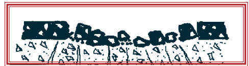
POTHOLE DUE TO BASE FAILURE
