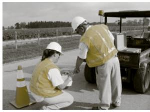
Contractors must purchase their own inertial profilers, and LADOTD will certify each one annually using a series of static and dynamic tests. The first calibrations were completed in May. Approval will be based on each profiler's ability to produce accurate IRI values on test strips predetermined by the department. Contractors must also be able to furnish a report with all data specifically requested by LADOTD.
