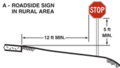
Figure 2A-2. Examples of Heights and Lateral Locations of Sign Installations
