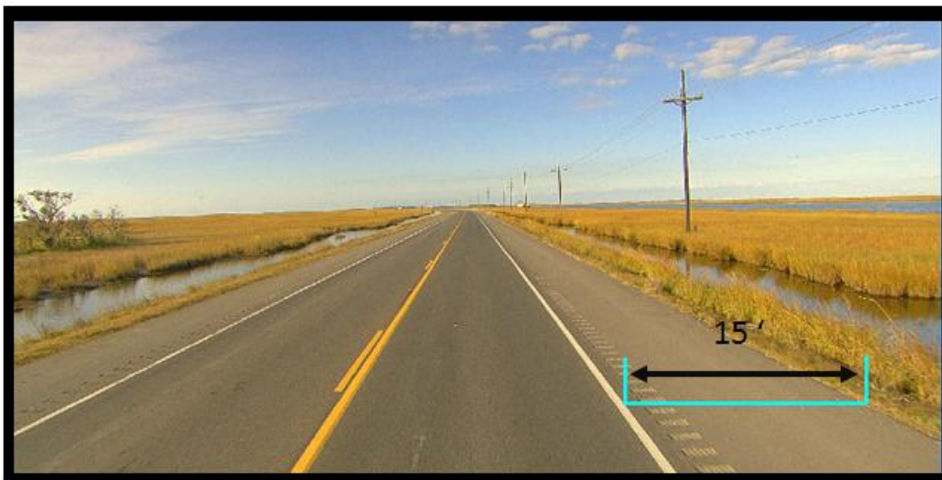
'Example of Shoulder Width Measurement'. The Louisiana Department of Transportation & Development ©2008
