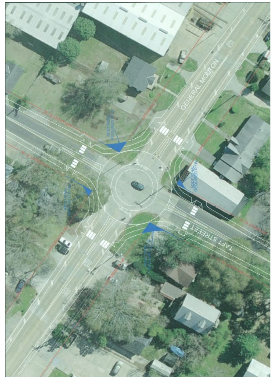
Proposed Roundabout Design General Mouton @ Taft St., Lafayette, LA
