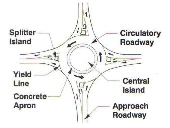
Roundabouts are designed to accommodate fire trucks and large vehicles. Large trucks may have to drive on the concrete apron around the central island in order to get through the roundabout.
