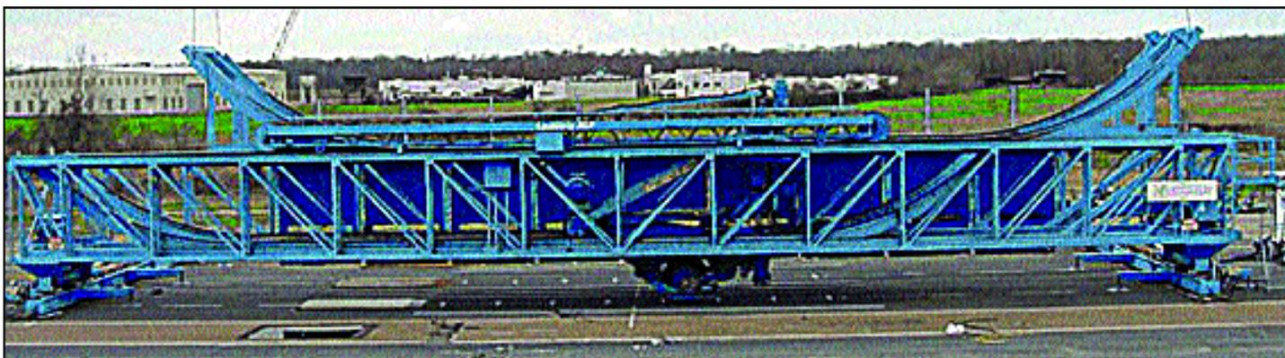
*Accelerated Loading Device at Pavement Research Facility*
