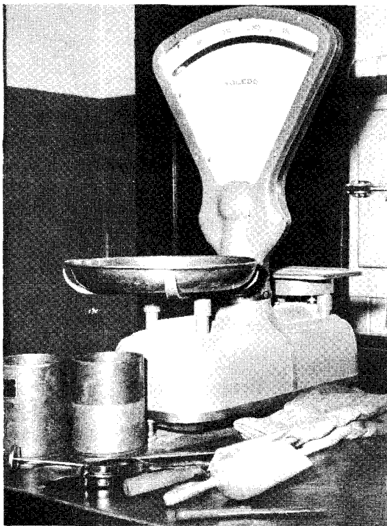
FIGURE 3 Apparatus for Weighing, Mixing and Molding Aggregate - Asphalt Mixture
