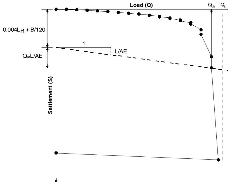
**Figure 1 Estimation of ultimate bearing resistance using Davisson (18) method (after Salgado (20)).**
