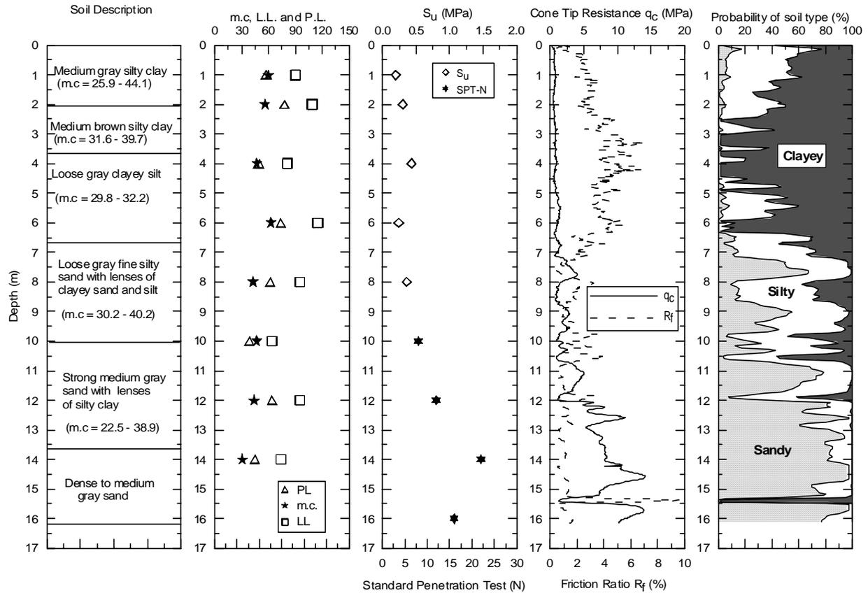
**Figure 2 Typical summary of geotechnical data for a tested pile.**
