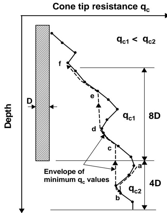
**Figure 3 Average cone tip resistance ( $q_{c,avg}$ ) in Schmertmann (14) method (from Abu-Farsakh and Titi, (25)).**
