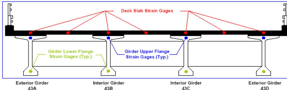
HPC SPAN NO. 43 - CROSS SECTION THRU MIDSPAN - LOOKING EAST
