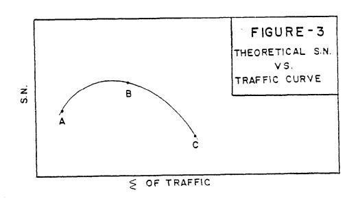
The skid numbers are more traffic dependent than they are time dependent. Thus, if for this study the first skid tests fell near Point A and the second near Point B, there would be an increase in the numbers. If instead, the first tests fell on or near Point B, and the second near Point C, then a decrease would be found.
