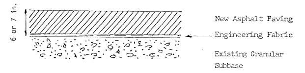
c. E.F. BETWEEN EXISTING ASPHALT PAVING AND NEW ASPHALT SURFACE
