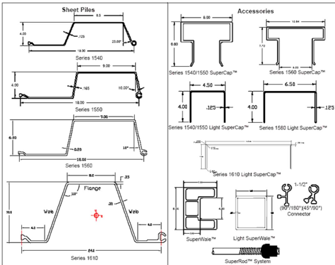
Figure 22 Superloc sheet pile geometry
