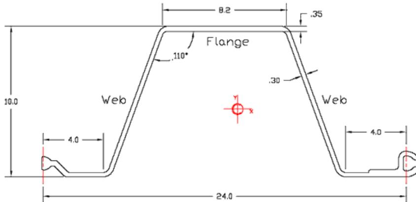
**Figure 24 Geometric properties of 1610 Superloc system**
