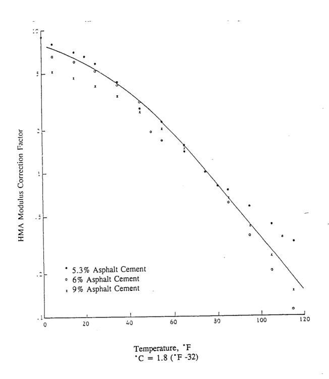
Figure 3. Relationship selected for modifying HMA modulus as a function of temperature
