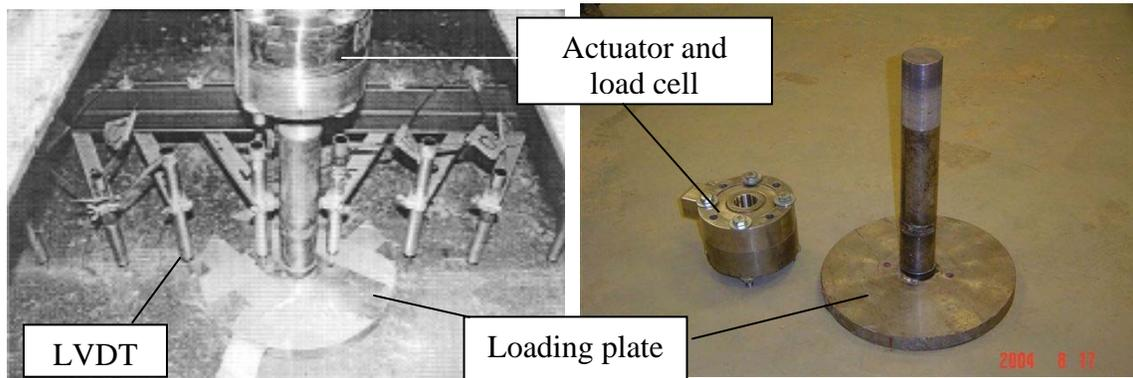
**b) Loading and rutting measurement**
