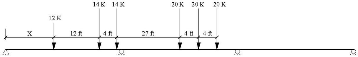
(b) Case 2 GVW=100 Kip with Max Tandem Load 28 Kip and Max Tridem Load 60 Kip
