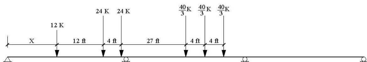
(a) Case 1 GVW=100 Kip with Max Tandem Load 48 Kip and Max Tridem Load 40 Kip
