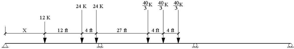
(a) Case 1 GVW=100 Kip with Max Tandem Load 48 Kip and Max Tridem Load 40 Kip
