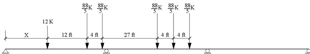
(c) Case 3 GVW=100 Kip with Uniformly Distributed Tandem and Tridem Loads.
