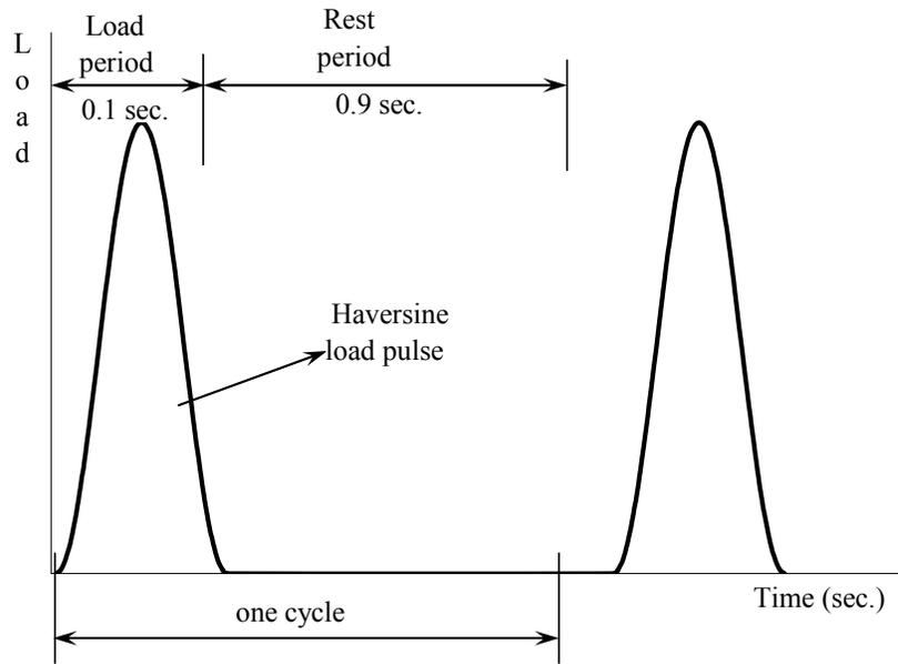
**Figure 11: Haversine load pulse used in RLT tests**
