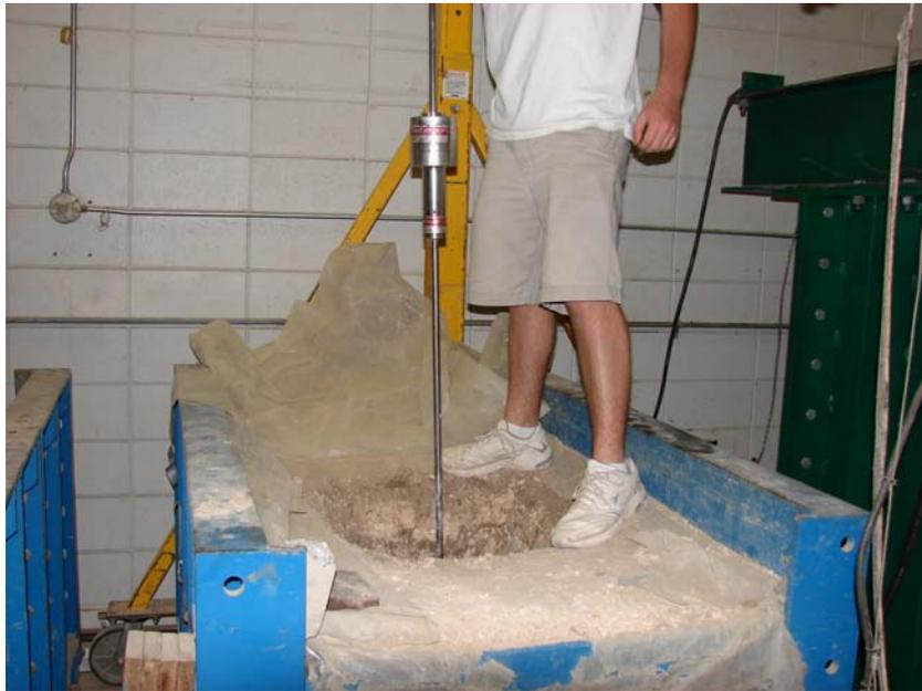
**Figure 9: DCP test conducted in the pit of a steel-frame box**
