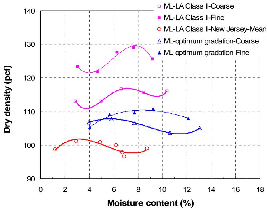
**Figure 13: Standard Proctor compaction curves for Mexican limestone with different gradations**
