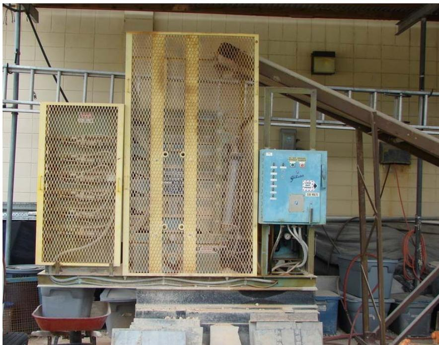
**Figure 5: Picture of shaker machine for sorting unbound aggregate**
