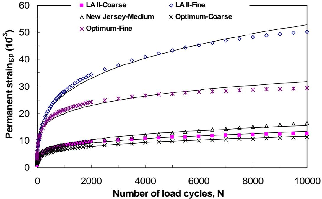
**Figure 23: Variation of permanent deformation with number of load cycles for Mexican limestone specimens with different gradations**
