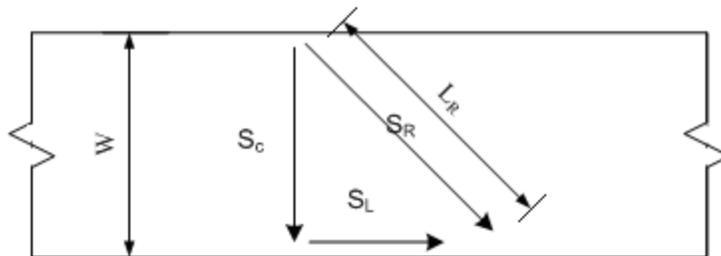
**Figure 3: Typical pavement flow-path gradient**
