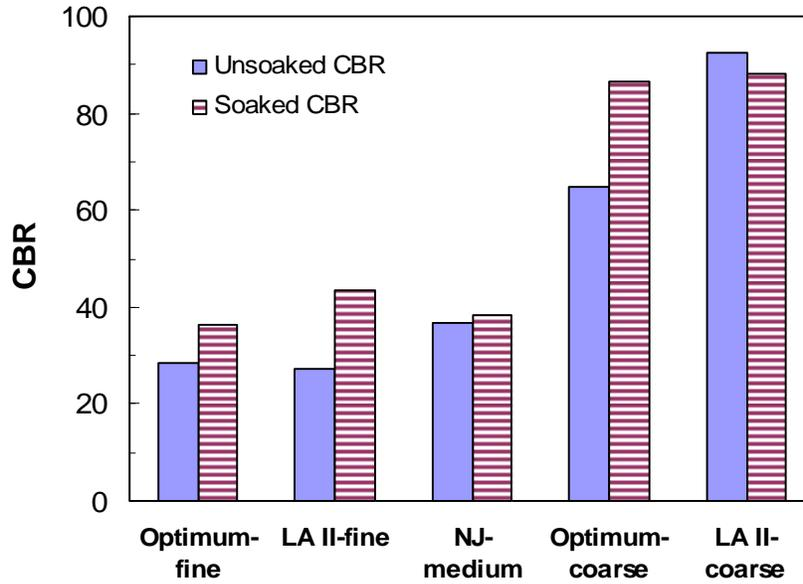
**Figure 17: CBRs at 0.1 inches penetration for Mexican limestone at different gradations**
