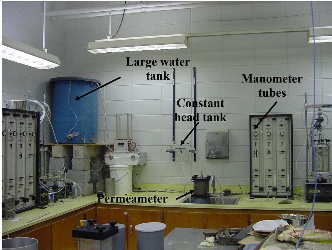
**Figure 7: Picture of setup for constant-head hydraulic conductivity test**
