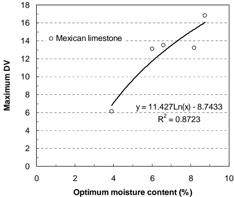
**Figure 16: Correlation between maximum DV values and optimum moisture contents determined from Standard Proctor tests for Mexican limestone with different gradations**
