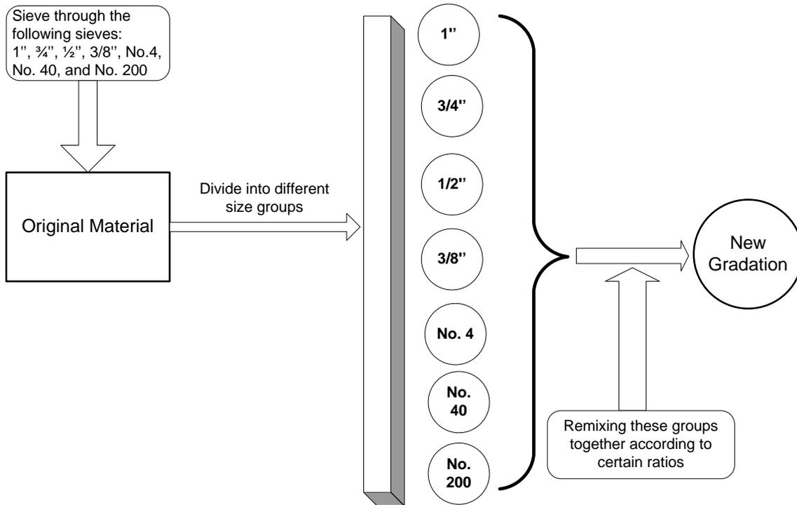
**Figure 4: Testing procedure to obtain different particle size gradations**
