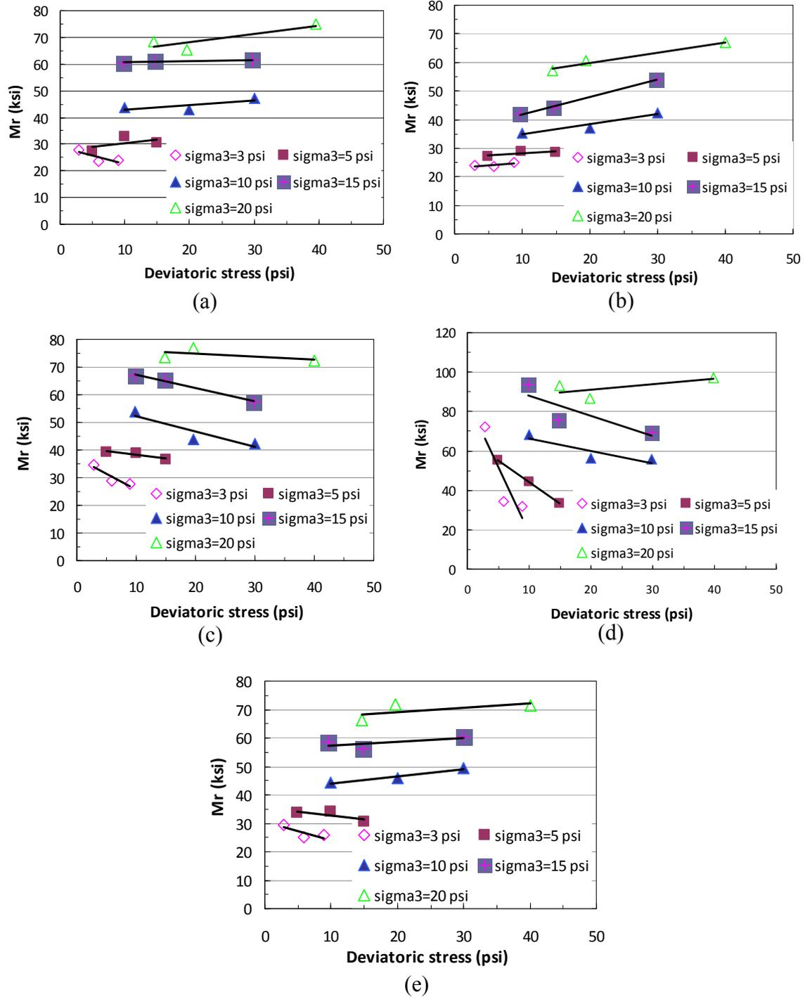
Figure 22: Resilient moduli of Mexican Limestone at various gradations at corresponding optimum compaction conditions: (a) LA II-coarse; (b) LA II-fine; (c) NJ-medium; (d) Optimum-coarse; and (e) Optimum-fine
