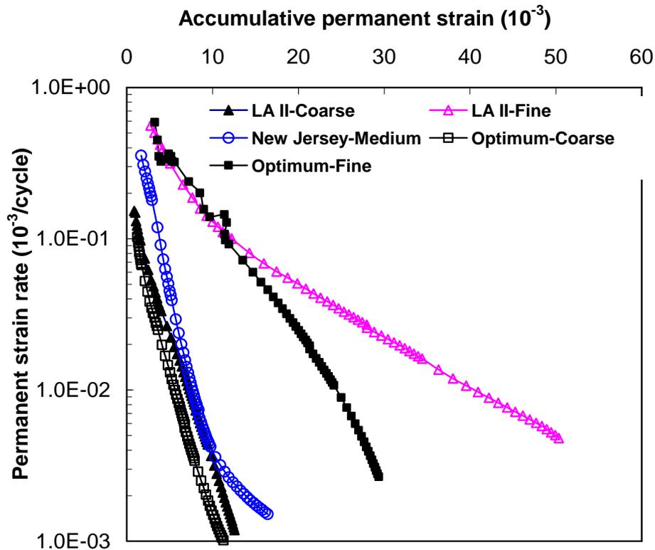
**Figure 24: Variation of permanent strain rate with accumulative permanent strain for Mexican limestone specimens with different gradations**
