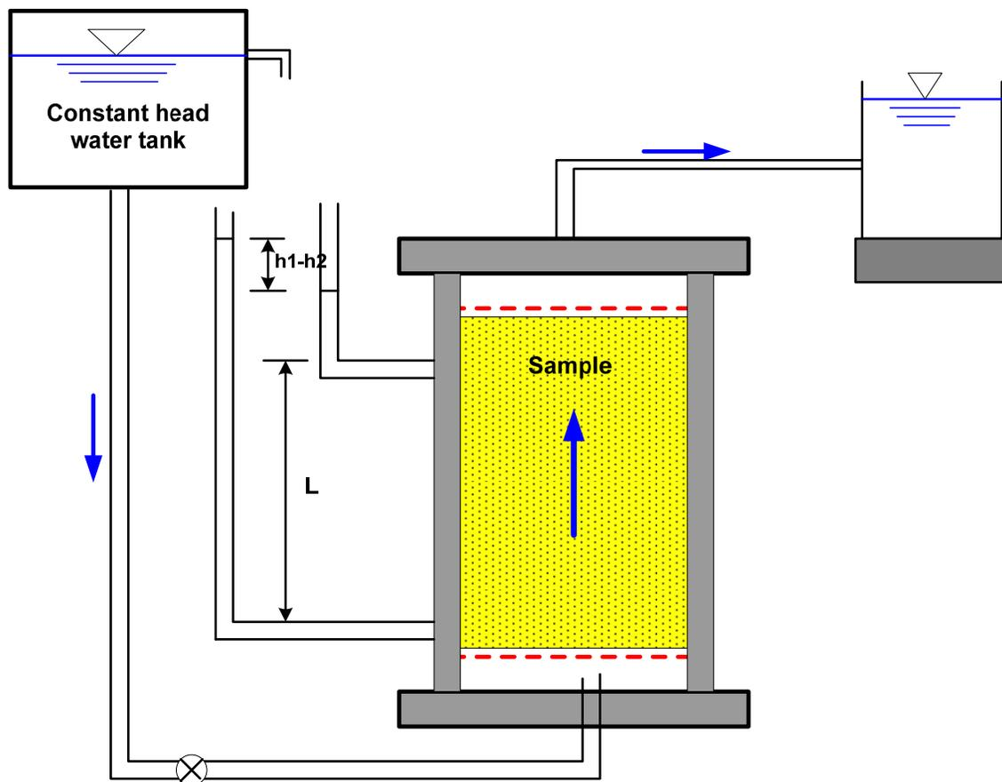
**Figure 6: Schematic diagram for set-up of constant-head hydraulic conductivity test**
