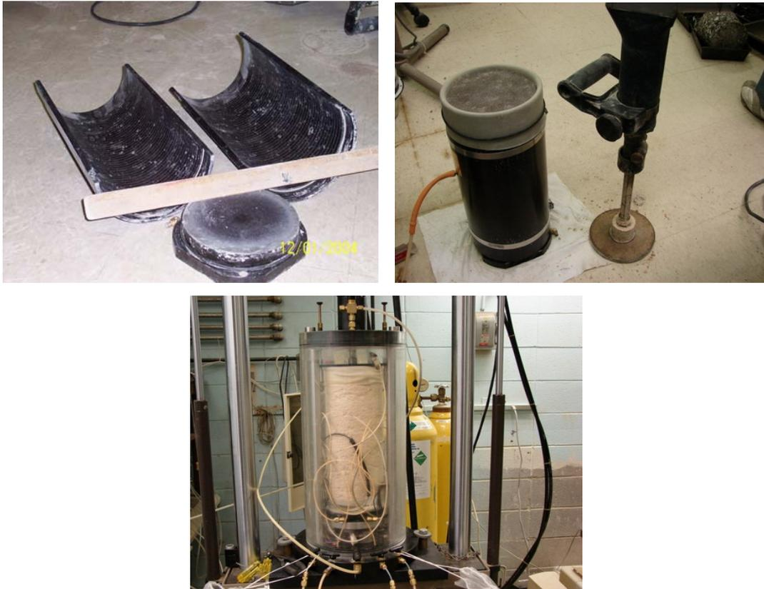
**Figure 10: Compaction of RLT test samples**
