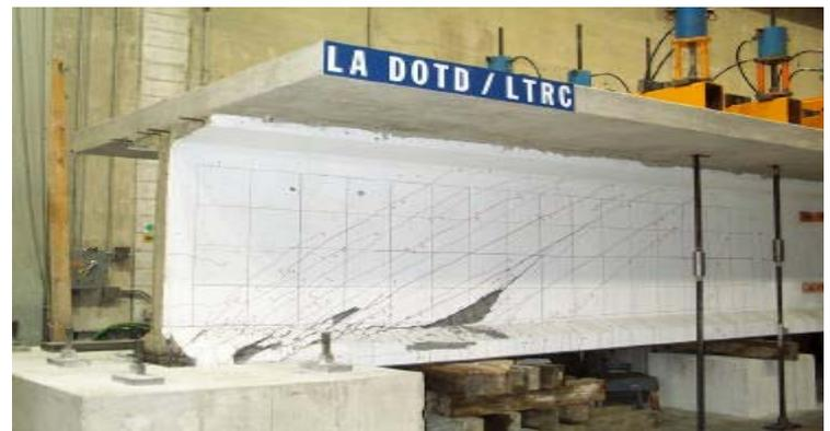
*Shear Test at CTL*
