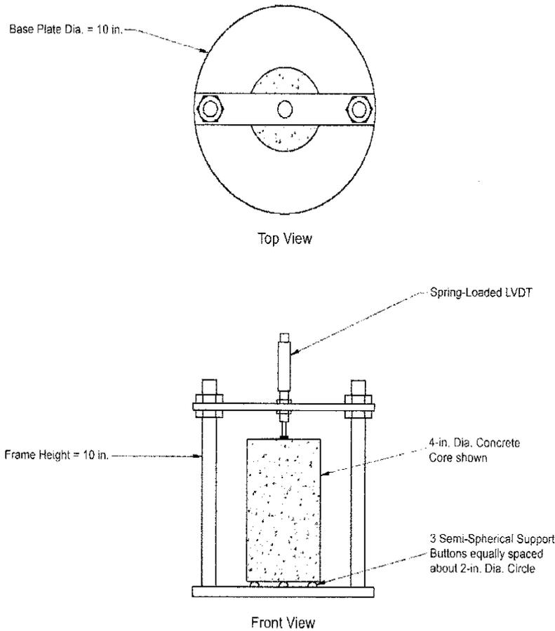
**Figure X1.1**—Schematic of a Measuring Frame
