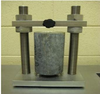
5. Place the frame with specimen into the water bath, and fill the water bath to 1 in. below from the specimen surface.
