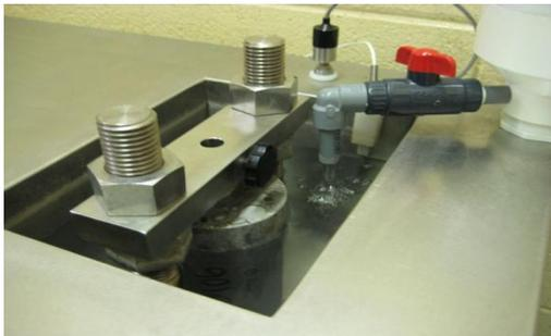
6. Fill the water level control reservoir (WLCR) by opening both valves. Pour water into the WLCR until water appears through the opposite valve. Close both valves. Place the WLCR in the back right corner of the cabinet with the 90° elbow in the water bath and open the valve. This must be full and open so that it supplies the water consistently to prevent the water loss due to the evaporation.
