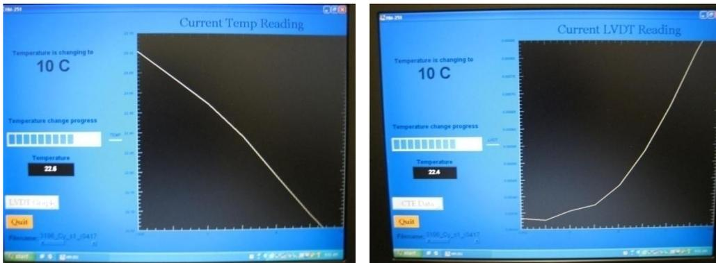
14. Testing is complete when the difference between the expansion CTE and contraction CTE is between 0.3 microstrains/C. The average CTE is then displayed.
