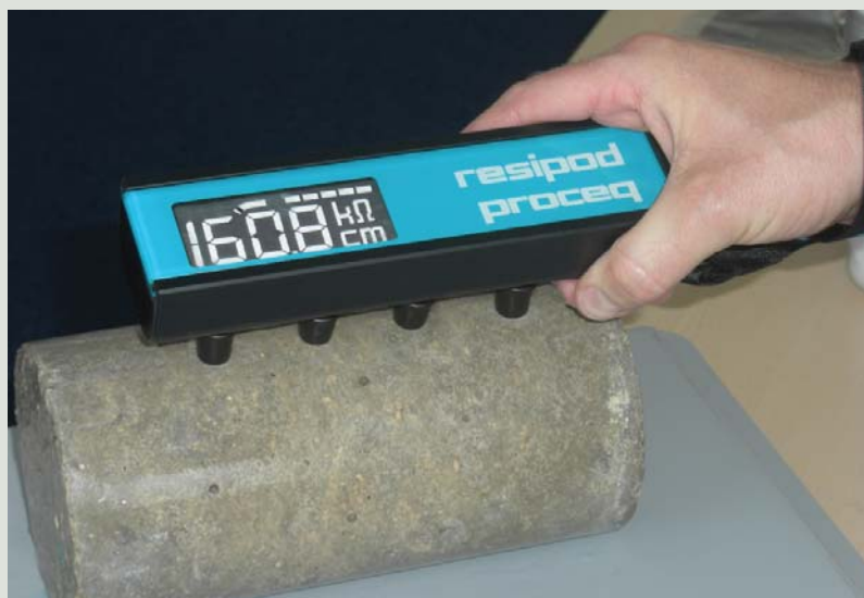
Surface resistivity meter
