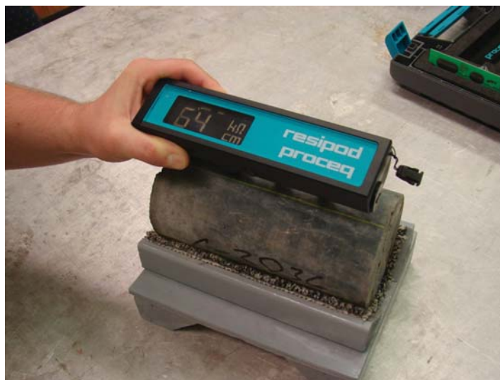
Surface resistivity test being conducted on a 4- x 8-in. cylinder
