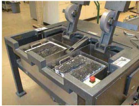
Figure 4 Hamburg LWT device
