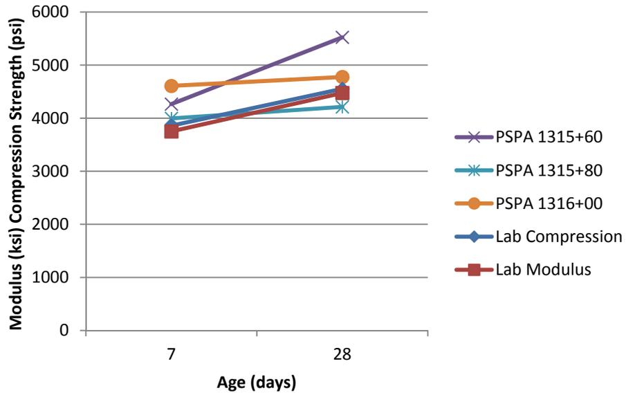
**I-49 section 2 PSPA seismic modulus compared to laboratory modulus and compression strength**
