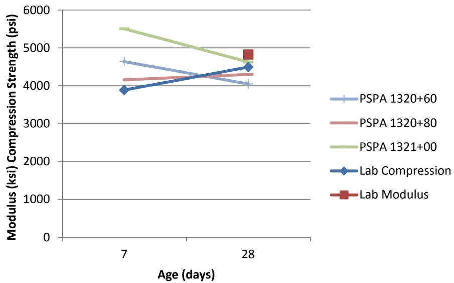
**I-49 section 3 PSPA seismic modulus compared to laboratory modulus and compression strength**
