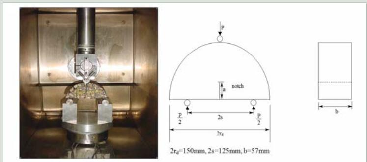
Semi circular bend test setup and specimen configuration
