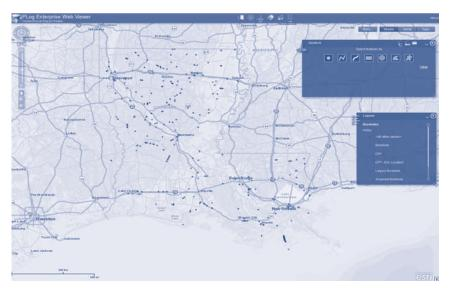
The web-based GIS map converts the DOTD geotechnical data into a valuable asset that can be reused over time. The map-based interface provides a simple and direct way for DOTD personnel and its consultants to find historical geotechnical data, generate reports, and ultimately get the data in a digital format so it can be re-used on future projects.
