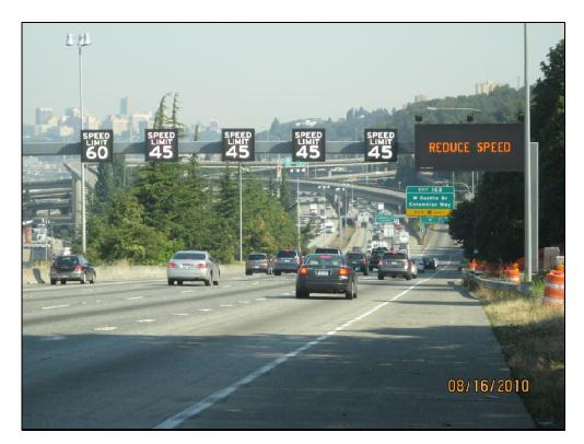
Figure 7 Example of variable speed limits
