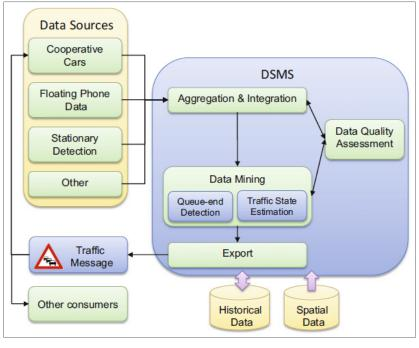
Figure 3 Overall architecture of data stream management system
