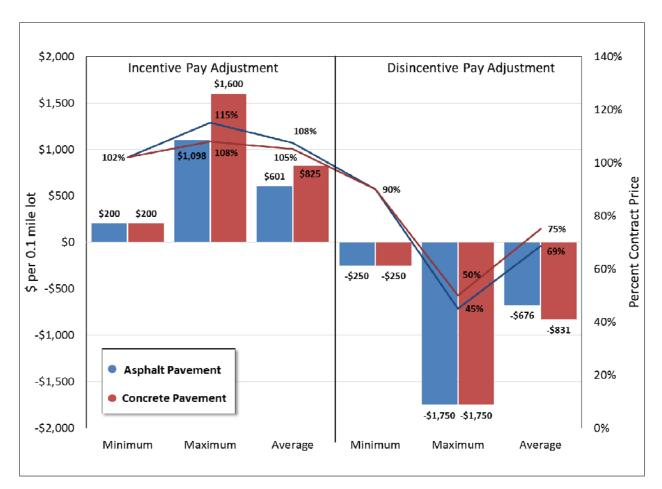
Figure 8 Comparison of asphalt and concrete incentives and disincentives for IRI-based specifications
