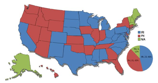
Figure 2 Smoothness specifications for concrete pavements by state
