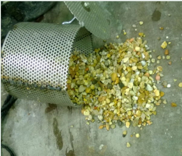
Figure 1 Washout test result for a No. 8 pea gravel mixture showing no cement paste
