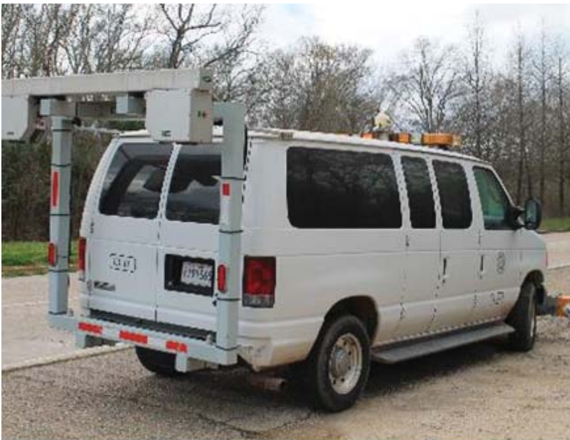
Figure 1 LTRC's Digital Highway Data Collection System
