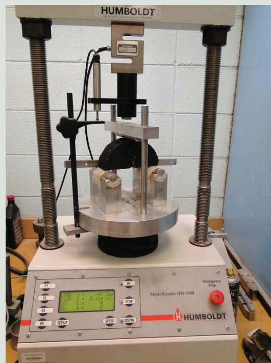
Figure 1 Marshall Load frame device
