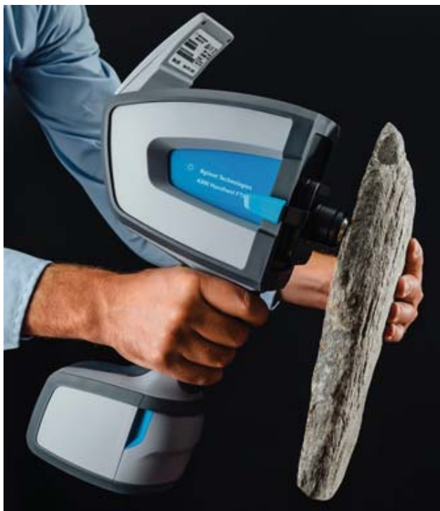
Figure 2 An Agilent 4300 Handheld FTIR Spectrometer
