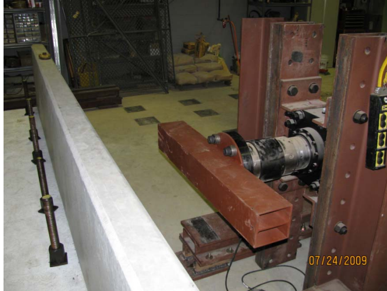
Figure 56 View of the ram with the metal box bolted to its head
