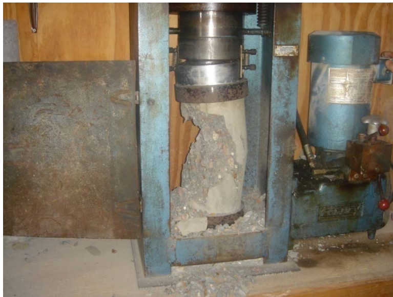
Figure 27 Determination of the compressive strength, f'_c , of a concrete cylinder
