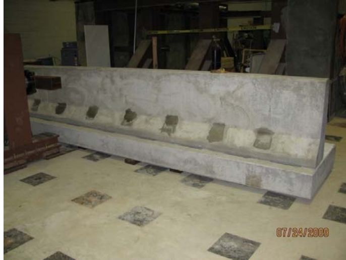
Figure 48 Front view of slab-barrier system after it was connected at the center
