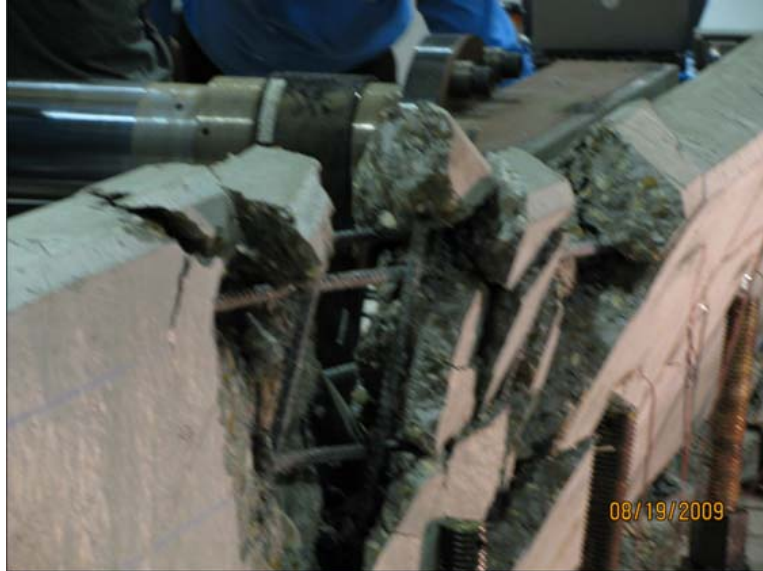
Figure 71 Hydraulic ram cracking top of barrier
