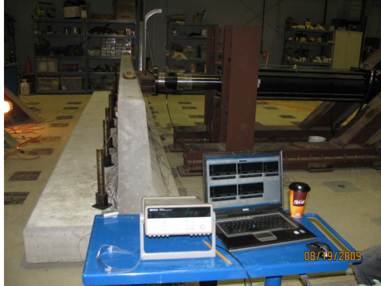
Figure 59 Laptop and data logger used in the test
