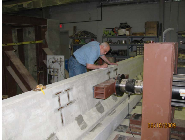
Figure 58 Ram in slight contact with the sloping face of barrier
