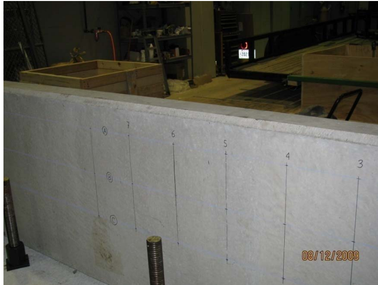
Figure 51 Marking up the barrier to place the strain gauges
