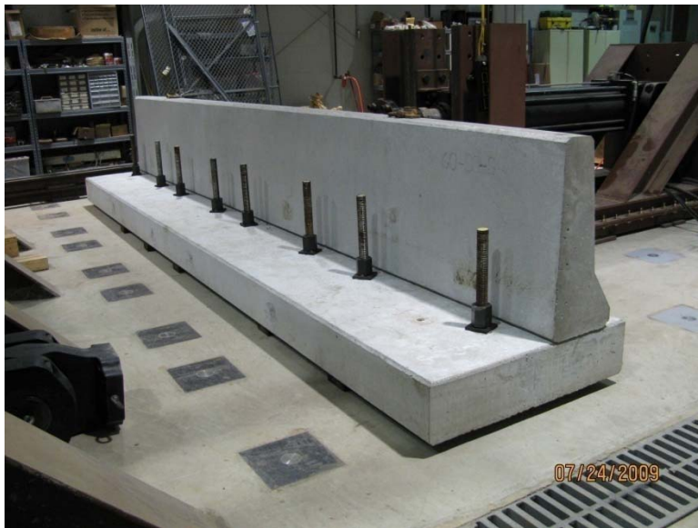
Figure 47 Rear view of slab-barrier system after it was connected at the center
