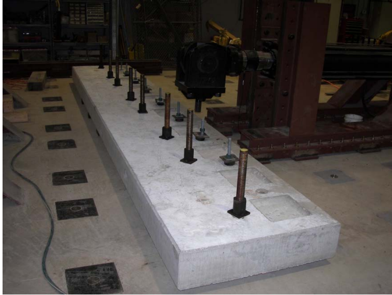
Figure 46 Anchoring the slab to the strong floor
