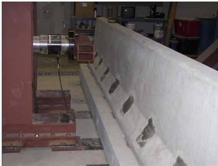
Figure 61 Lining of the hydraulic ram head against sloping face of barrier
