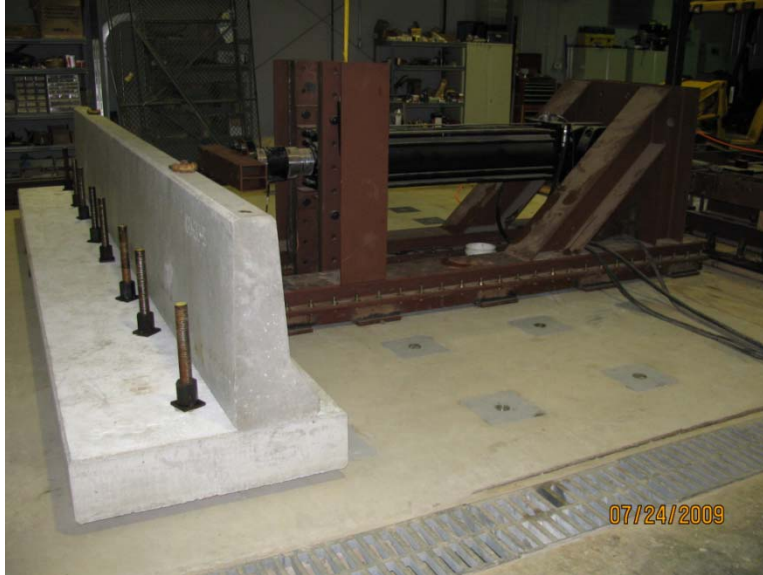
Figure 54 Hydraulic ram used in transverse load application
