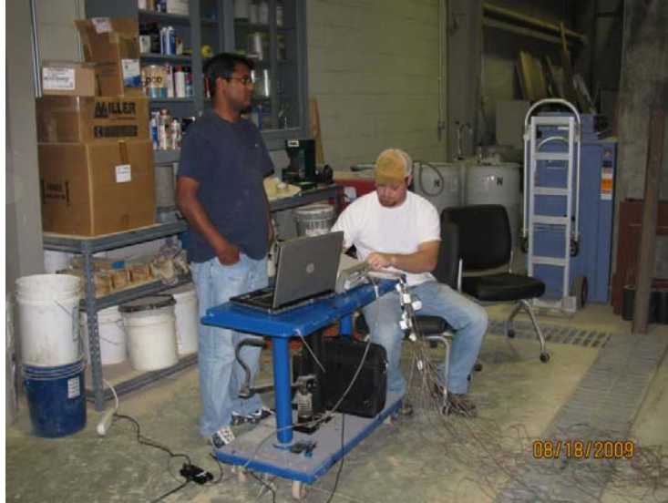
Figure 53 Strain gauge wires being connected to the data logger
