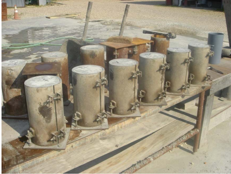
Figure 26 Concrete cylinders made at the plant
