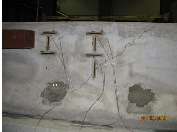
Figure 64 Diagonal cracks developing on sloping face of barrier
