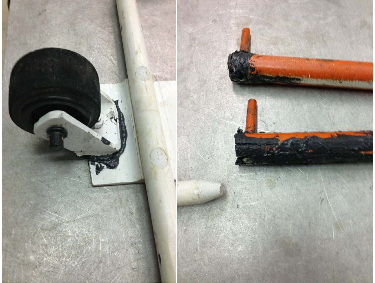
Figure 11 Examples of epoxy repair to the fiberglass track
