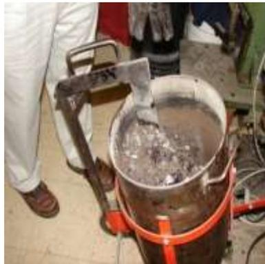
Asphalt binder and aggregate mixed together
