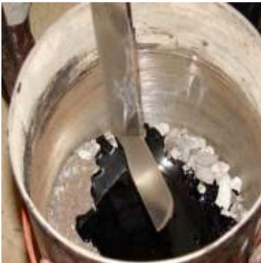
Asphalt binder added to prepared aggregate blend
