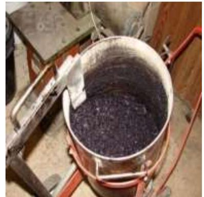
Asphalt mixture after mixing
