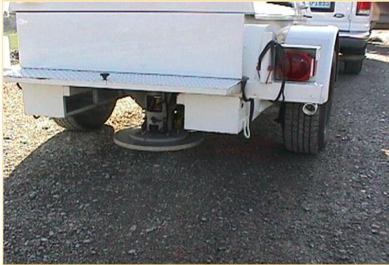
**(a) FWD testing using a circular plate**
