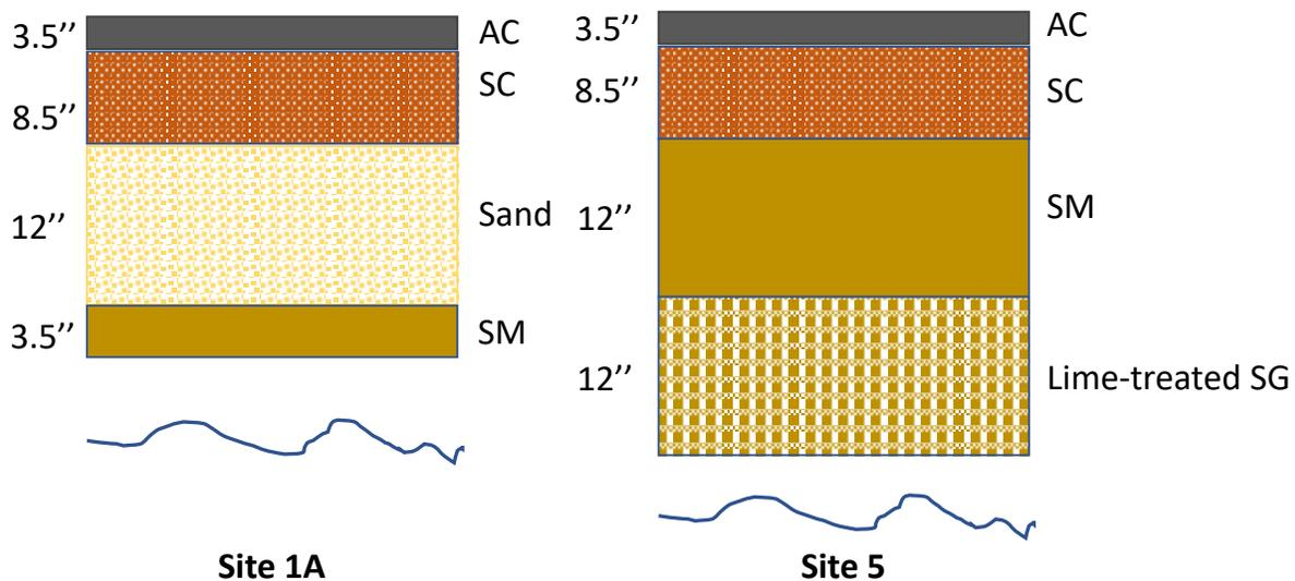
AC: asphalt concrete; SC: soil-cement base course; SG: subgrade; SM: selected materials (soil that meet DOTD’s usable soil criteria)
