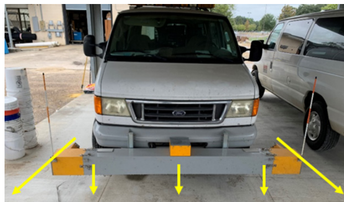
Figure 1 LTRC's 5-point rut bar system
