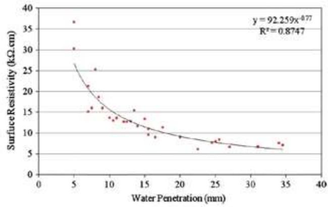
**Figure 5. Relationship between EN 12390-8 water penetration and SR for all mixtures [46]**
