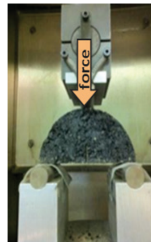
Figure 4 Semi-circular bend test setup
