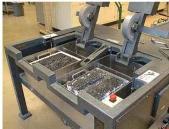
Figure 2 Loaded wheel tracking test device - AASHTO T 324
