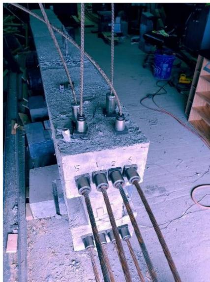
**Figure 35. Placement of the mono-strand jack**
