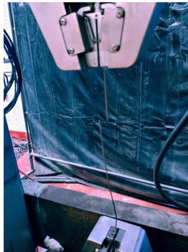
(b) Tensile failure of the wire
