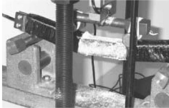
Sherif et al. studied the use of SMAs to self-post-tension concrete beams by taking advantage of the grout's heat of hydration [8]. They examined the temperature increase due to heat of hydration of four commercial grouts and explored the feasibility of activating NiTiNb alloys. A recovery stress of over 500 MPa was accomplished after cooling to ambient temperature.
