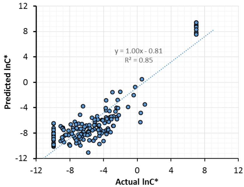
Figure 11: Predicted versus actual  $\ln(\text{TC}^*)$  for AST interlayer over soil-cement base
