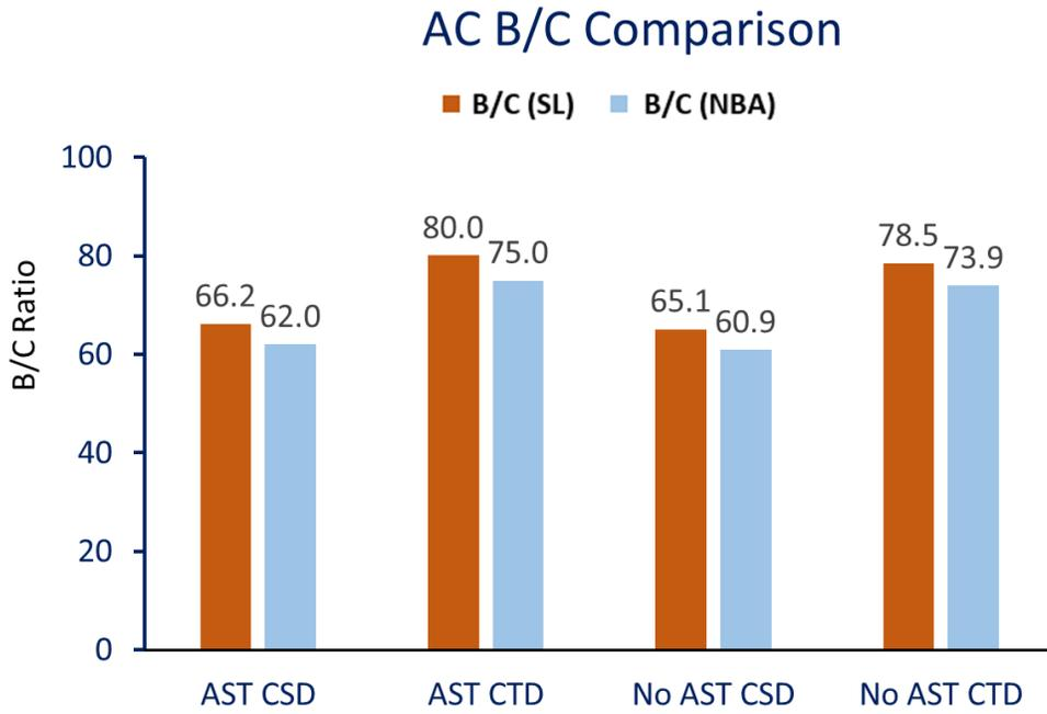
**Figure 223: Alligator cracking B/C ratios comparison**
