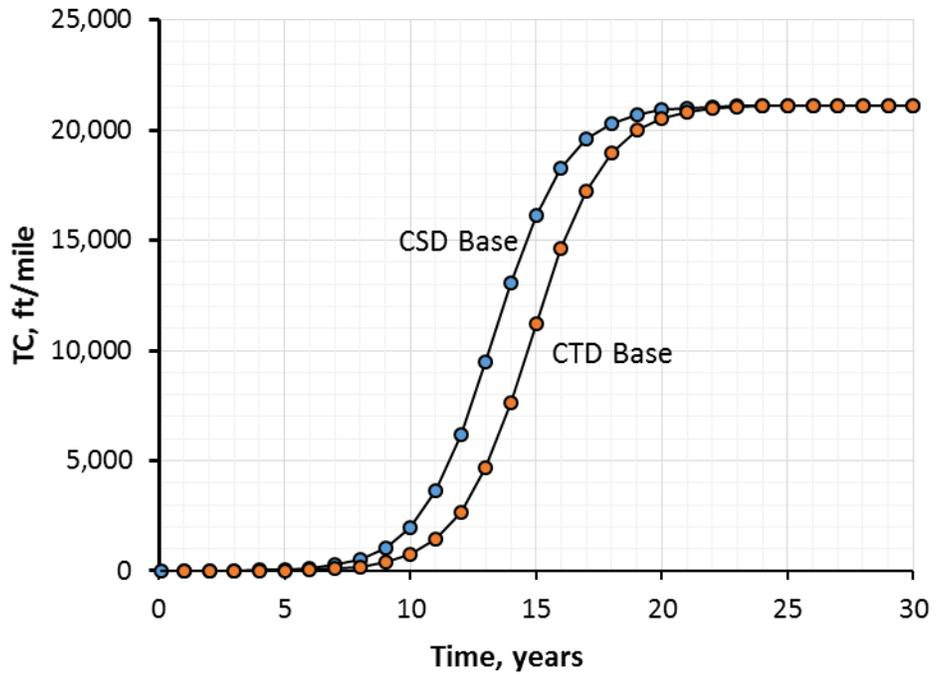
Figure 22: TC model behavior for no AST interlayer over soil-cement base
