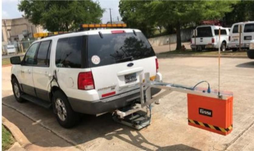
The equipment typically consists of a control unit, monitor, and two dipole bowtie (ground coupled) antennae operating at center frequencies of 900 MHz and 1.6 GHz. The setup can perform up to 16 scans per ft. at 10 mph, which results in a scan about every 1 in. The data are collected at the posted speed limit with a maximum of 55 mph, although the speed varies based on traffic and stops. A typical GPR acquisition setup is presented in Table 2.
